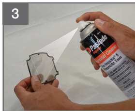
3 Use Paslode Cordless Tool Cleaner or mild detergent and water to clean filter
