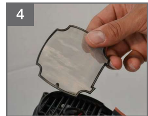
4 Ensure filter is completely dry before reinstalling
