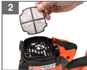
2 Tap filter gently to remove dust and debris
