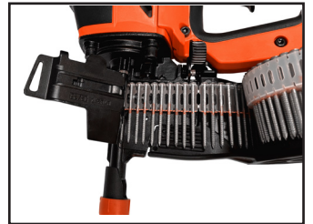
Insert nails into nose area
