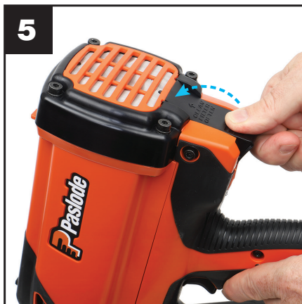
5 To close - Push forward, then down to lock fuel door
