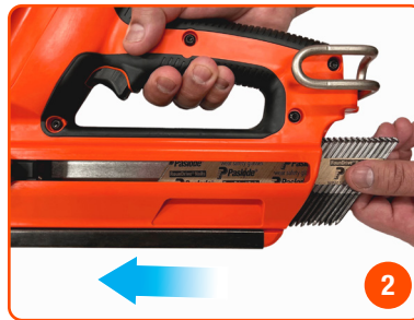
Pull the follower up past the last nail. Avoid letting the follower slam forward into the nails.
