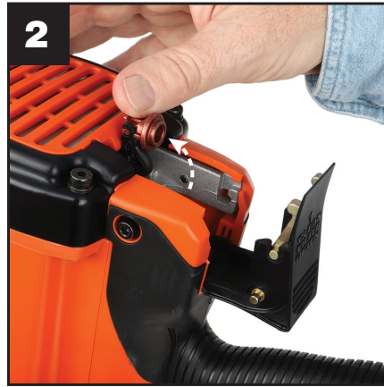
2 Raise fuel tube block assembly, it will lock in up position
